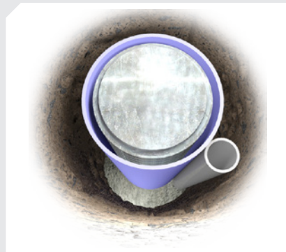
Cross-section of the free length of the anchor with an injection pipe
