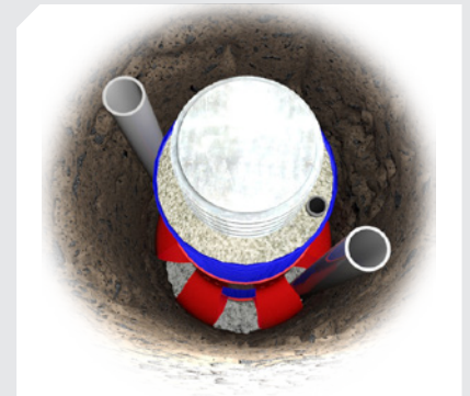
Cross-section of the bond length of the anchor with an injection pipe
