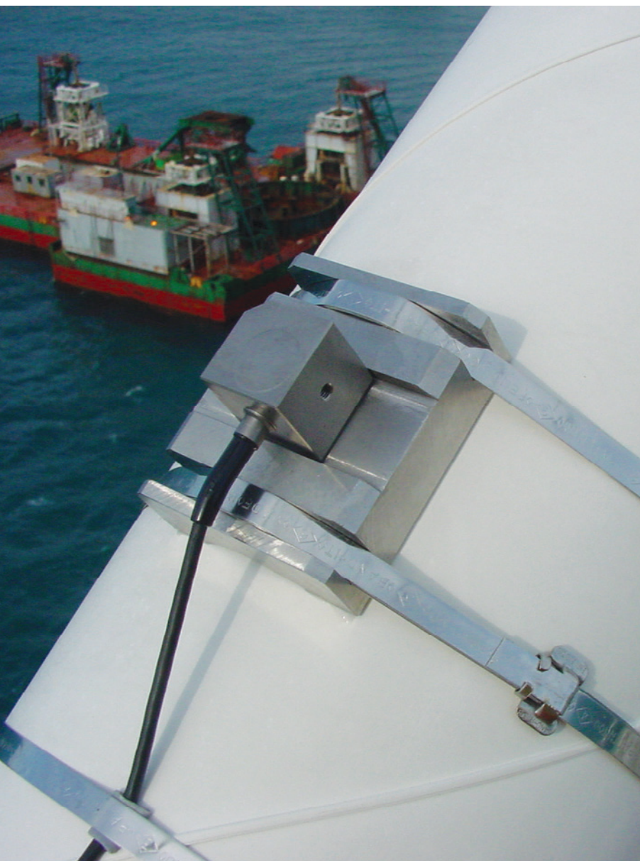
Stay cable fitted with an accelerometer
